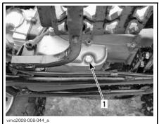
LH SIDE OF ENGINE 1. Drain plug
